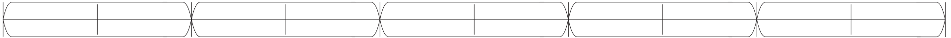
1/5 Cut Bank (2" Wide with 3/8" Extension, 1/2" Inset on Left & Right of Tab Bank)
