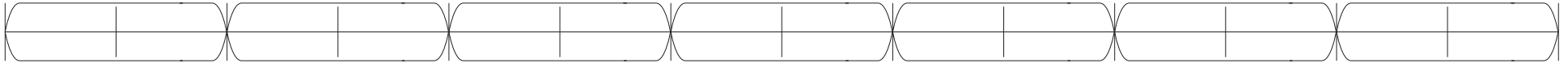
1/7 Cut Bank (1 3/8" Wide with 3/8" Extension, 1/2" Inset on Left & Right of Tab Bank)
